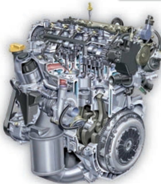
Forced-induction, downsized engines – such as this Corsa turbo unit – represent the future for IC powertrains, especially in hybrid applications and range extender vehicles
