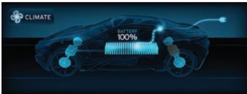
In pure electric mode, the i8 concept can go for 35km before calling upon the three-cylinder petrol engine. Expect the production version of the i8 sports car to achieve an even greater EV driving range
