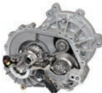
The single-speed eAxe Family 2, with a disconnect system feature
