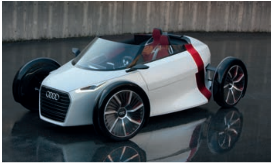
The 1+1 Urban concept (above) shows a new EV direction for Audi. The 480kg EV has a 90kg Li-ion battery and two electric motors producing 15kW of continuous power output and 47Nm of torque
