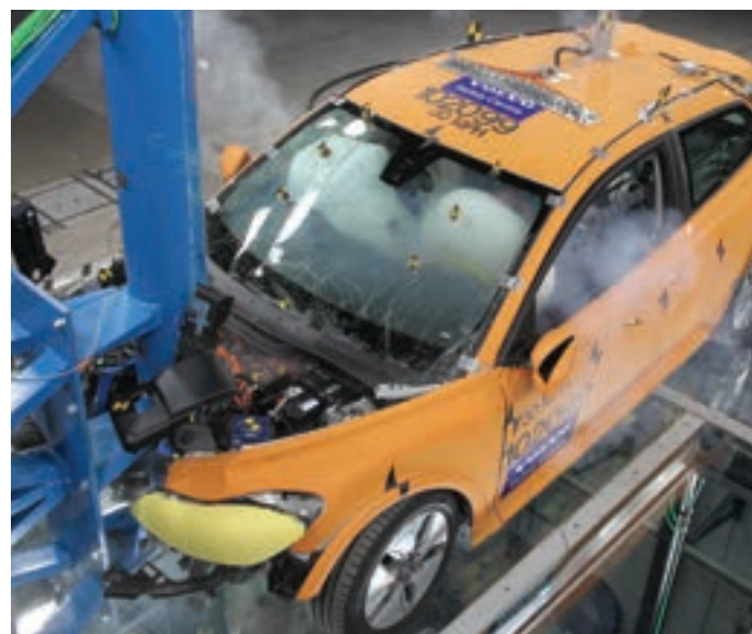
A Volvo C30 Electric undergoes a 30mph pole test. The EV's Li-ion batteries survived as they are installed in the propshaft tunnel and fuel tank space
